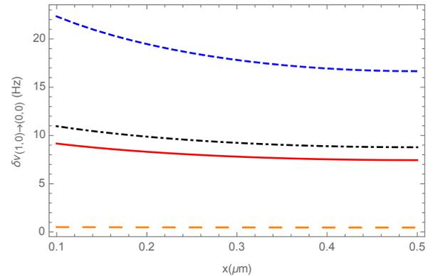
FIG. 3: Shift  $\delta\nu$  (in Hz) of the H hyperfine transition ( $F = 1, m_F = 0$ )  $\rightarrow$  ( $F = 0, m_F = 0$ ) (in Hz), versus the minimum atom-mirror separation  $x$  (in micron). The atom is placed inside a metallic cavity of width  $a = 1$  micron at room temperature, in a magnetic field  $B = 0.01$  G. The thickness of the metallic layer is 5 micron. The four curves, from top to bottom, are for a cavity made of Ag, Al, Au and Pt, respectively.
