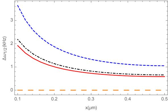
FIG. 4: Half-width  $\Delta\omega_{1/2}$  (in kHz) of the H hyperfine transition ( $F = 1, m_F = 0$ )  $\rightarrow$  ( $F = 0, m_F = 0$ ) (in Hz), versus the minimum atom-mirror separation  $x$  (in micron). The atom is placed inside a metallic cavity of width  $a = 1$  micron at room temperature, in a magnetic field  $B=0.01G$ . The metallic layers have a thickness  $w=5$  micron. The four curves, from top to bottom, are for a cavity made of Ag, Al, Au and Pt, respectively.
