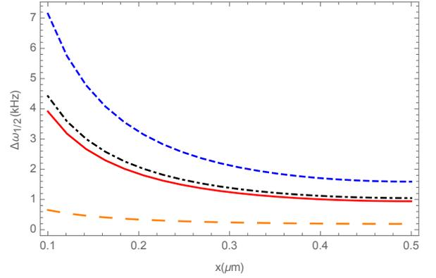
FIG. 6: Half-width  $\Delta\omega_{1/2}$  (in kHz) of the H hyperfine transition ( $F = 1, m_F = 0$ )  $\rightarrow$  ( $F = 0, m_F = 0$ ) (in Hz), versus the minimum atom-mirror separation  $x$  (in micron). The atom is placed inside a metallic cavity of width  $a = 1$  micron at a temperature  $T = 70$  K (RRR=10), in a magnetic field  $B=0.01G$ . The metallic layers have a thickness  $w=5$  micron. The four curves, from top to bottom, are for a cavity made of Ag, Al, Au and Pt, respectively.
