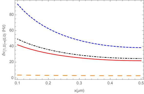
FIG. 5: Shift  $\delta\nu$  (in Hz) of the H hyperfine transition ( $F = 1, m_F = 0$ )  $\rightarrow$  ( $F = 0, m_F = 0$ ) (in Hz), versus the minimum atom-mirror separation  $x$  (in micron). The atom is placed inside a metallic cavity of width  $a = 1$  micron at a temperature  $T = 70$  K (RRR=10), in a magnetic field  $B=0.01G$ . The metallic layers have a thickness  $w=5$  micron. The four curves, from top to bottom, are for a cavity made of Ag, Al, Au and Pt, respectively.
