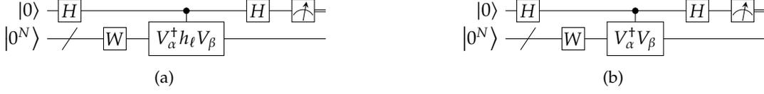
Figure 1: Quantum circuits implementing the Hadamard-test for estimating (a)  $\text{Re}(\langle \Phi_\alpha | H | \Phi_\beta \rangle)$  and (b)  $\text{Re}(\langle \Phi_\alpha | \Phi_\beta \rangle)$ .
