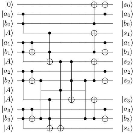
Fig. 2: Proposed out-of-place QCLA for the case of adding two 4 bit values  $a$  and  $b$ .
