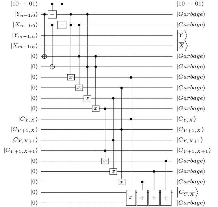
(b) Quantum bilinear interpolation circuit for scaling down by a value  $n$ .
