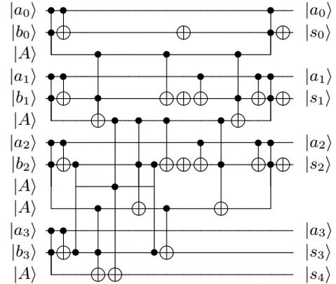
Fig. 3: In-place QCLA for the case of adding two 4 bit values  $a$  and  $b$ .
