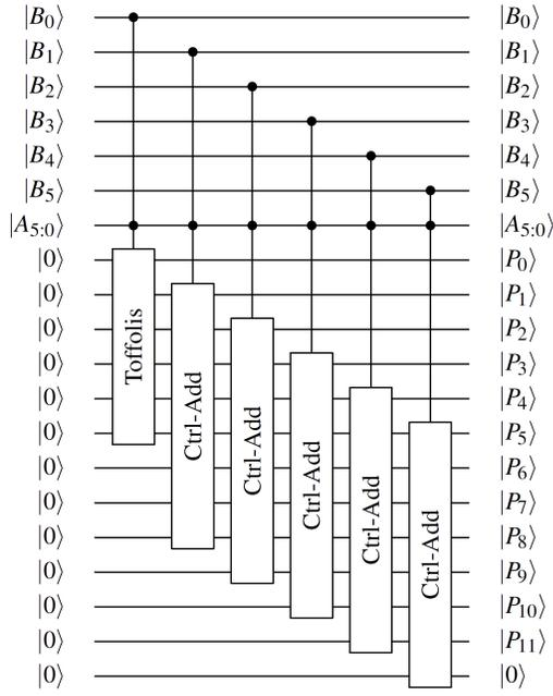
Fig. 5: Example of the proposed quantum integer multiplication circuit for the multiplication of two 6-bit inputs  $|A\rangle$  and  $|B\rangle$ .  $|P\rangle$  is the product of the values in  $|A\rangle$  and  $|B\rangle$ .
