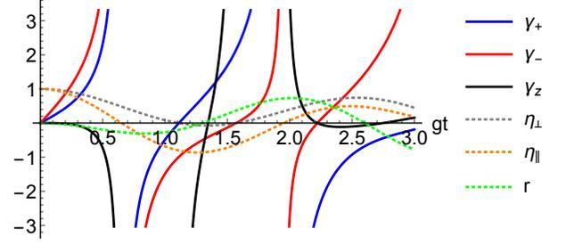
FIG. 3. The time behavior of rates corresponding to the Jaynes-Cummings master equation, Eq. (50), and the functions  $\eta_\perp(t)$ ,  $\eta_\parallel(t)$  and  $r(t)$ , Eq. (51), for the environment initially in the number state  $|1\rangle$ . All three rates  $\gamma_+(t)$ ,  $\gamma_-(t)$  and  $\gamma_z(t)$  are negative for some time intervals and diverge at isolated points in time.
