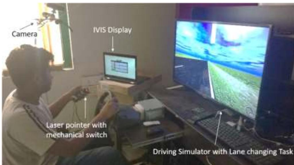
Figure 5. Participant performing a secondary task using laser tracker with a mechanical switch
