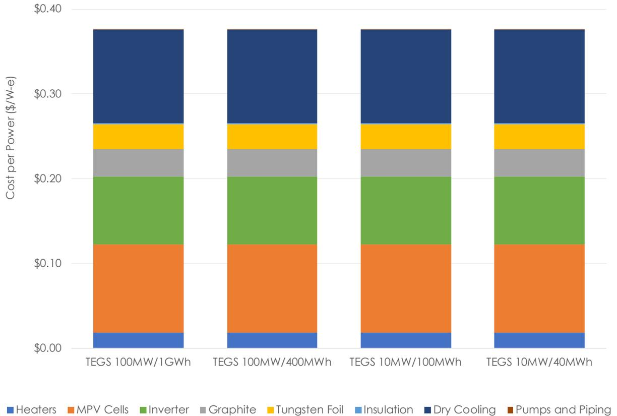
**Figure 3:** CPP for the power block at multiple scales. Due to the decoupled power and energy components of the TEGS system, this cost does not scale with size of the storage system and changes minimally with varying power scales.
