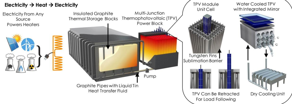
**Figure 1:** Proposed TEGS concept using graphite storage blocks, a molten tin heat transfer fluid, and a multijunction TPV heat engine.
