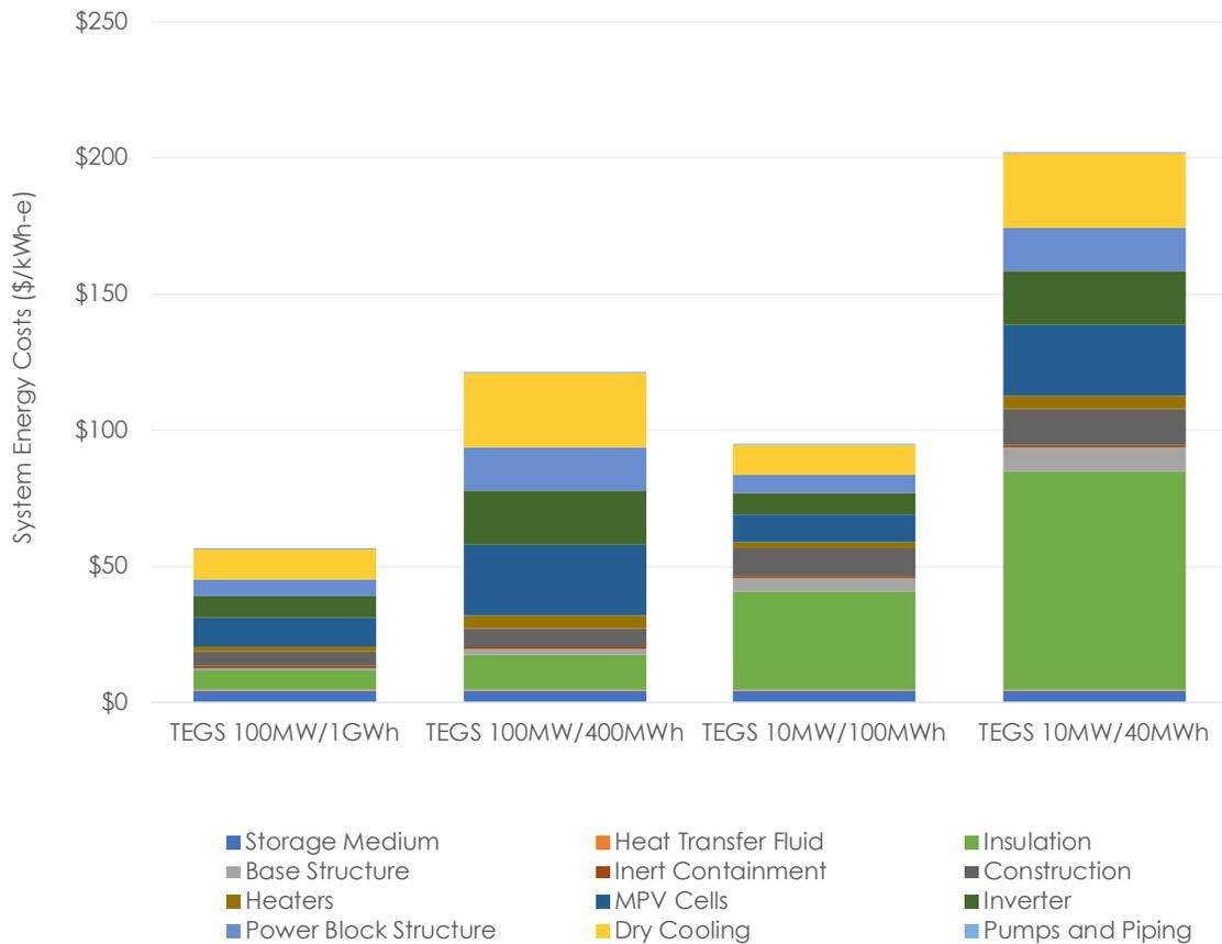
**Figure 4:** Total cost of energy incorporating the Cost per Energy and Cost per Power into a system energy cost for the four proposed cases.
