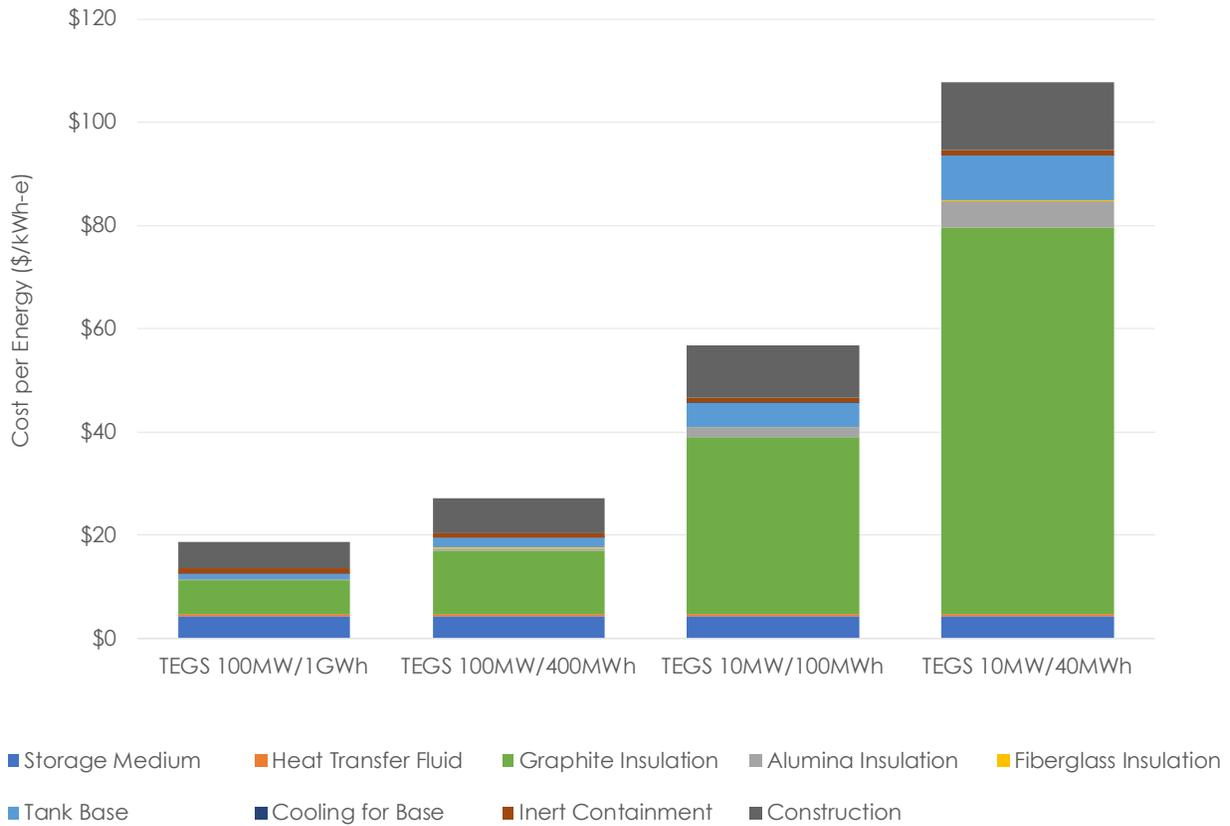
**Figure 2:** Cost per Energy at multiple scales for the energy storage component of TEGS
