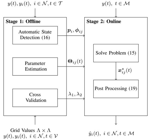
Figure 1. Overall disaggregation process: Stage 1 (Offline) and Stage 2 (Online). For all  $i, j, t$  we denote by  $\Theta_{ij}(t) = [w_i, l_i, s_i(t), a_{ij}, b_{ij}, o_i, m_{ih}]^T$  the vector of the parameters.
