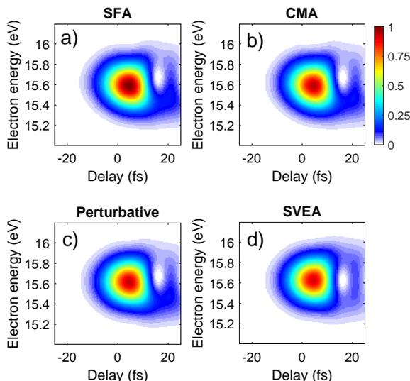
**Figure 3.** Effect of the consecutive approximations introduced ((a) SFA, (b) CMA, (c) perturbative and (d) SVEA) for the case of a third order dispersion on the IR pulse. The SVEA is responsible for the major distortion of the SB shape, resulting in an up-down symmetrization. This effect is observed only for what concerns the dispersion of the IR pulse and not for a dispersed XUV radiation.
