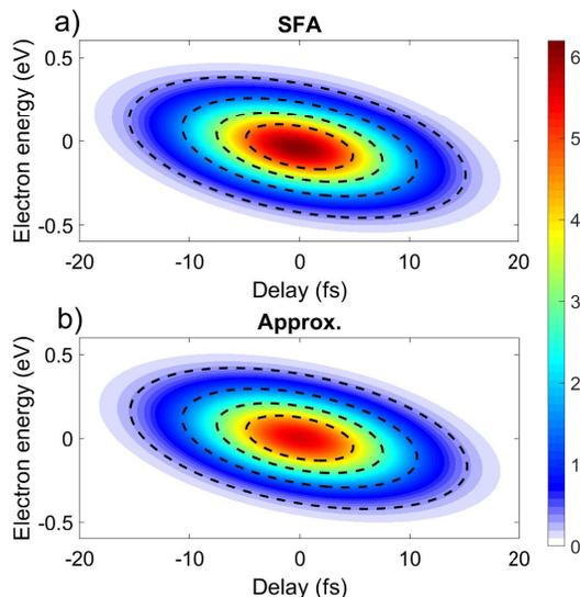
**Figure 4.** Comparison between  $SB^+$  computed with SFA calculations (a) and with the approximated model of (13) (b). The approximated model correctly reproduces the SFA results, with only a little discrepancy for what concerns the signal amplitude. In both panels the dashed black ellipses are computed using equation (15). They correctly match the shape of the SB.
