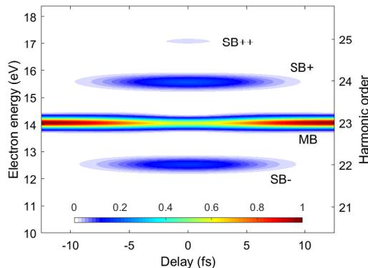
**Figure 1.** Example of a single-harmonic spectrogram computed with (1). The XUV pulse has a bandwidth of 0.4 PHz (about 5.9 fs duration), centered around the 23<sup>rd</sup> harmonic of 800-nm radiation. The IR has a bandwidth of 0.3 PHz, corresponding to a pulse of 7.8 fs, and an intensity of  $5 \cdot 10^{11}$  W/cm<sup>2</sup>. Both pulses have no dispersion. The noble gas considered in the simulation is neon.
