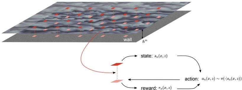
**Fig. 1 Diagram of the SciMARRL setup.** Agents are distributed evenly along the wall, with each agent obtaining state information wall-normal height  $h^m$  away from the wall, computing the reward at the wall and supplying in to the policy  $\pi$  to obtain actions  $a$  for the next time step.
