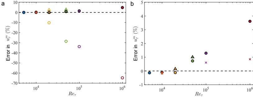
**Fig. 3 Errors in the friction velocities.** (a) Error in time-averaged wall-shear stress obtained from the VWM (empty) and LLWM (filled) for various Reynolds numbers. Circles indicate the standard grid with  $\Delta_y = 0.05$  and triangles indicate refined cases. (b) Zoomed in version of (a) for LLWM with error in EQMW (crosses) for three Reynolds numbers.
