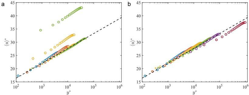
**Fig. 4 Predicted mean velocity profiles for turbulent channel flow.** Mean velocity profiles for the (a) VWM cases and (b) LLWM cases shown in figure 3. Dashed line is  $u^+ = 1/\kappa \log(y^+) + B$  for  $\kappa = 0.41$  and  $B = 5.2$ . The two largest Reynolds number cases for VWM are omitted as the velocity profiles are outside the plotted range.
