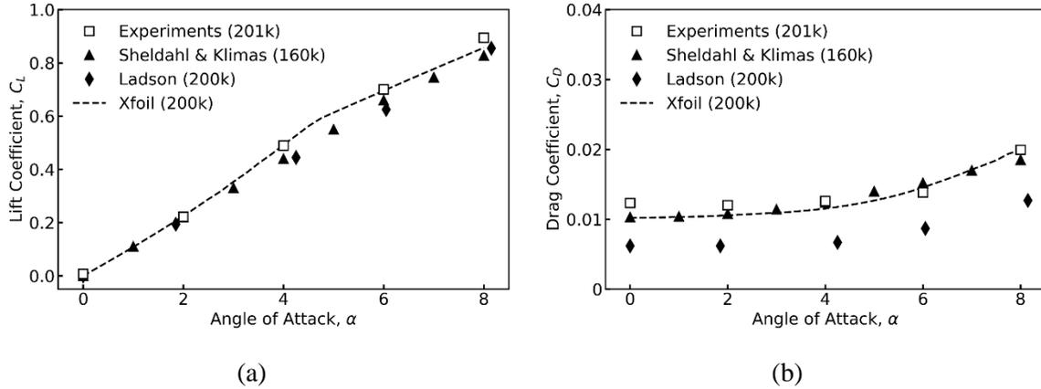
Figure 3. Comparison of measured aerodynamic coefficients for NACA 0012 airfoil, with XFOIL calculations (Drela 1989) and data from the literature (Ladson 1988, Sheldahl and Klimas 1981)
