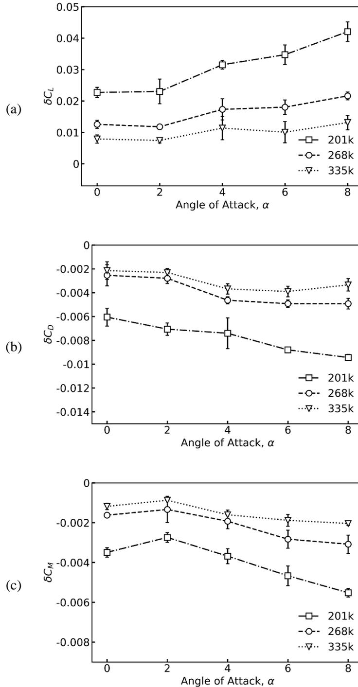
Figure 6. Effect of Reynolds number on (a) Lift (b) Drag (c) Pitching Moment for sawtooth DBD – DCA actuator.
