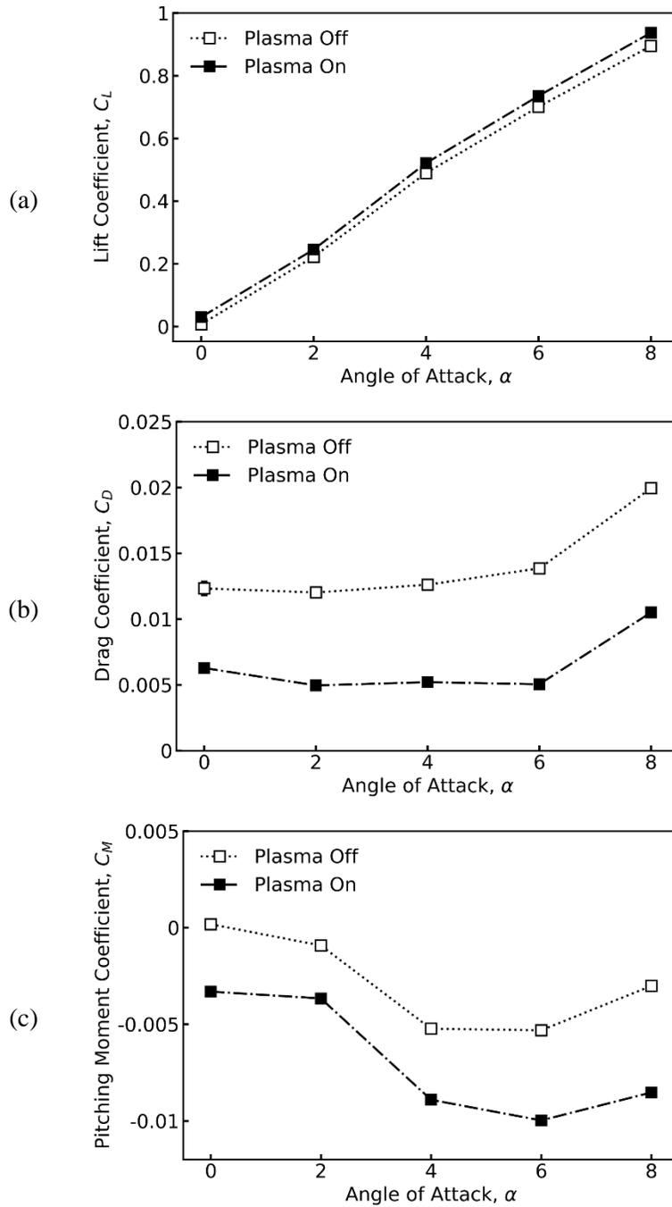
Figure 5. Aerodynamic characteristics (a) Lift (b) Drag (c) Pitching moment with/without plasma actuation at  $U_\infty = 15$  m/s. DBD - DCA is operated at  $\varphi_{p-p} = 18$  kV,  $\varphi_{bias} = 1.25$  kV,  $\varphi_{DC} = -15$  kV and  $f = 2$  kHz.
