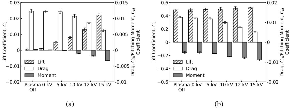
Figure 4. Aerodynamic performance at different  $\phi_{DC}$  potentials for two different angles of attack (a)  $0^\circ$  and (b)  $4^\circ$  ( $U_\infty = 15$  m/s), DBD - DCA is operated at  $\phi_{p-p} = 18$  kV,  $\phi_{bias} = 1.25$  kV and  $f = 2$  kHz
