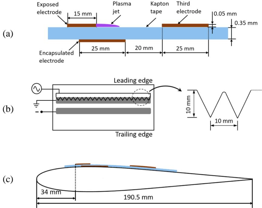
Figure 2. DBD – DCA actuator mounted on NACA 0012 airfoil (a) dimensions of the plasma actuator, (b) geometry of the sawtooth electrode pattern, and (c) actuator position on the airfoil.
