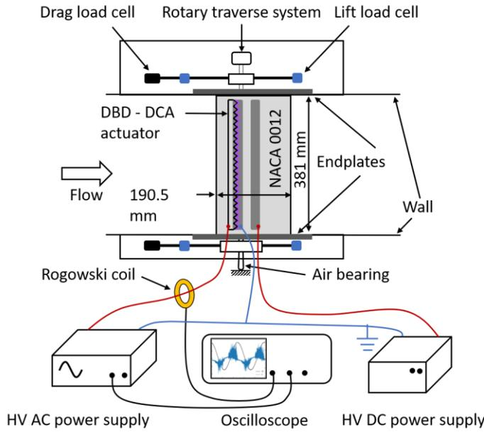
Figure 1. Schematic of the experimental setup for the lift, drag, and pitching moment measurements on the airfoil with sawtooth DBD – DCA actuator.
