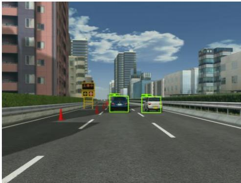
Fig. 1. Recognition results displayed to drivers, in which vehicles were recognized and pylons were not recognized.
