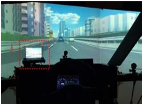
Fig. 2. Head-up display applied for the presentation of the results.
