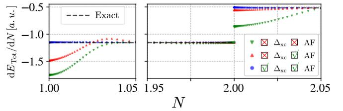
FIG. 4. Comparison of the derivatives of the energy with respect to the particle number  $N$  for three different models evaluated at a randomly chosen external potential: the first model uses only fractional densities, the second incorporates the exact xc shift in the loss function, and the third one uses a non-differentiable AF, in addition to the exact xc shift and the fractional densities.
