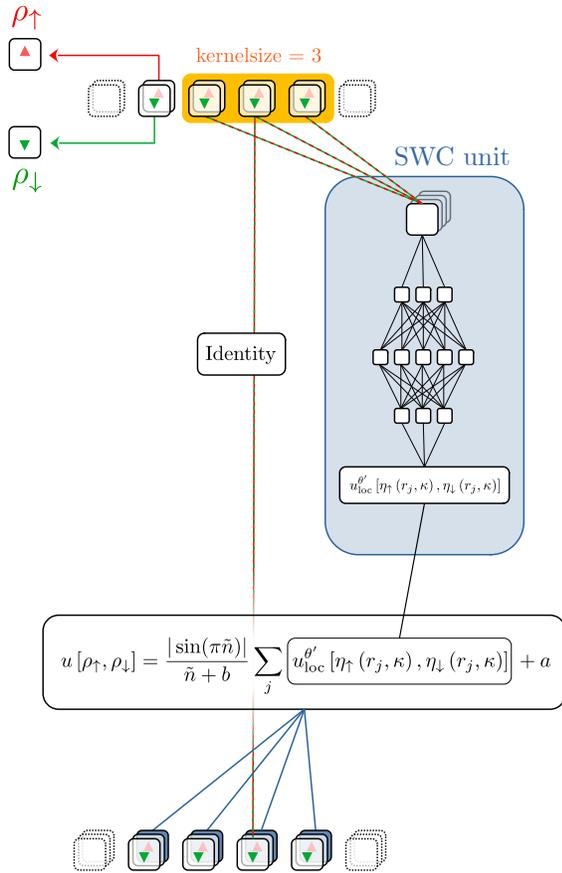
FIG. 3. Integration of the non-differentiable auxiliary function  $u[\rho_\uparrow, \rho_\downarrow]$  as a third channel to the basic SWC unit. The input data contains two channels for both spin-densities  $\rho_\uparrow$  and  $\rho_\downarrow$  respectively.
