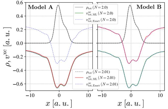
FIG. 5. Comparison between the predicted jump of the xc potential at  $N = 2$  for Model A and Model B (as explained in the main text). The results correspond to the same external potential used in Fig. 1.
