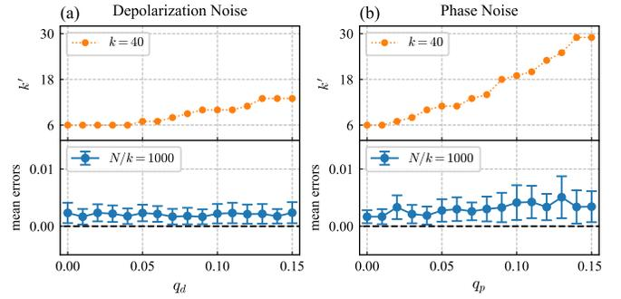
FIG. 4. The performance in the presence of noises. The measurement times needed in each period  $k'$  versus the noise strength under (a) depolarization noises and (b) phase noises. Mean errors and stds with our BPE-AL algorithm under (c) depolarization noises and (d) phase noises. Here,  $N/k = 1000$  with  $k = 40$ , and the estimated phase is  $\phi = 2.7624$ .
