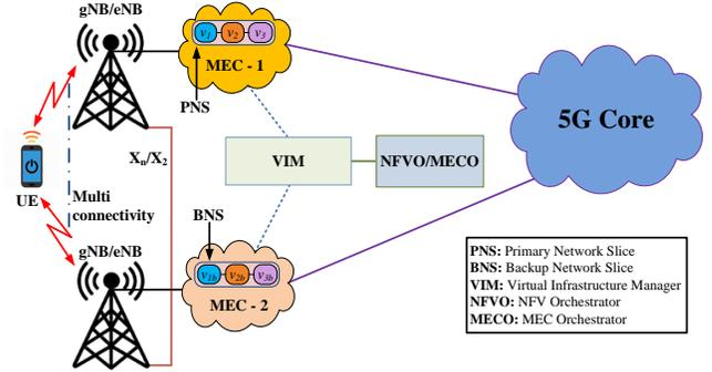
Figure 1: Multi-connectivity and MEC-enabled 5G network reference architecture.
