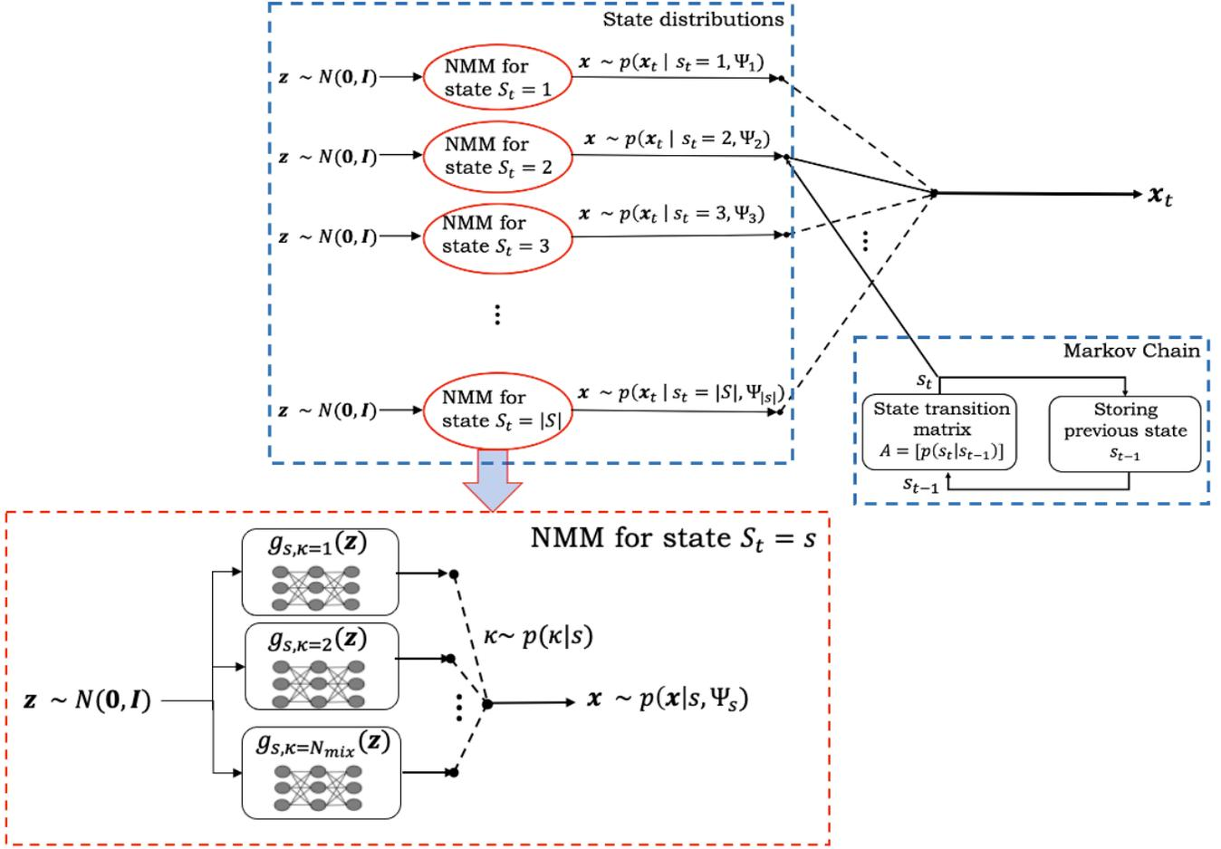
Fig. 1: Schematic of the NMM-HMM architecture. The architecture inside a single NMM model for a given state  $S_t = s$  is also shown in an expanded view at the bottom of the figure using red dotted line.
