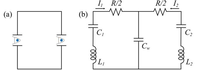
FIG. 1. (a) Schematic of two harmonically bound ions connected with a wire. (b) Equivalent circuit model of two ions coupled with a wire. The ion motion is modeled as inductance  $L_i$  and capacitance  $C_i$  while the current  $I_i$  corresponds to the ion velocity [15]. The coupling wire has ohmic resistance  $R$  and capacitance  $C_w$  to the rest of the trap.
