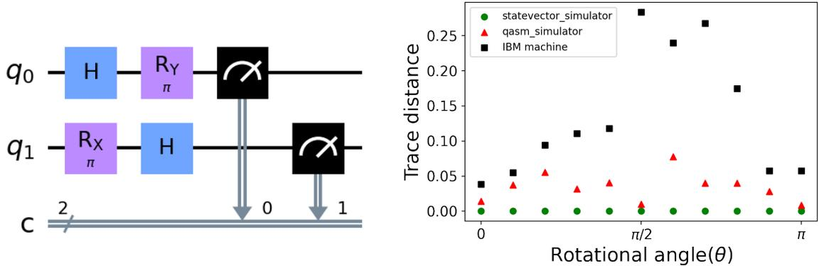
Figure 5: Trace distance between the true and the reconstructed state for the shown quantum circuit as a function of different rotational angles in  $R_x$  and  $R_y$  gates for the three backends in Qiskit: *statevector\_simulator*, *qasm\_simulator* and *IBM machine*.
