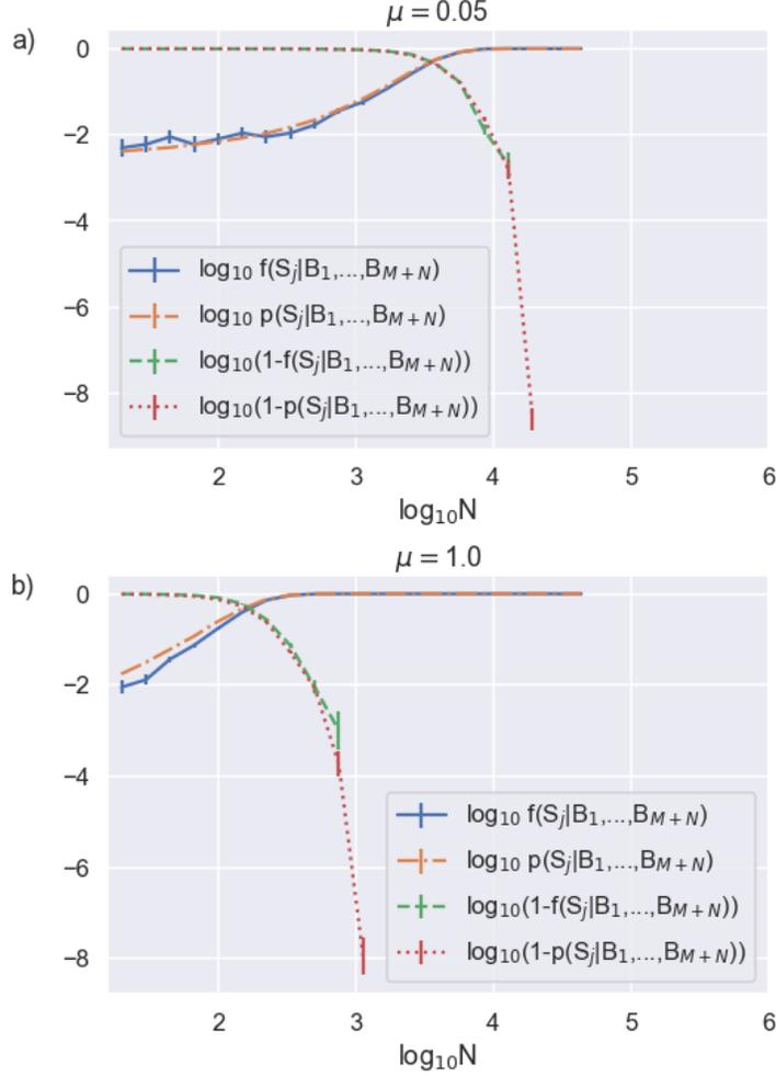
FIG. 2. Bob’s required data record length needed to determine synchronization for two different channel transmissions of (a)  $\eta = 0.05$ , corresponding to  $\mu = 0.05$  and (b)  $\eta = 1$ , corresponding to  $\mu = 1$ . We also show the probability of not obtaining synchronization, which better highlights transition to high-certainty synchronization.
