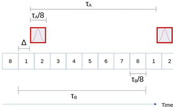
FIG. 1. Illustration of the relative times used in the QKD protocol. Here, the signal (red) straddles bins 1-2 due to an offset of  $\Delta$ , and we do not consider bins 3-8. We take  $\tau_A = \tau_B$ , which is approximately correct for a short enough data subset.
