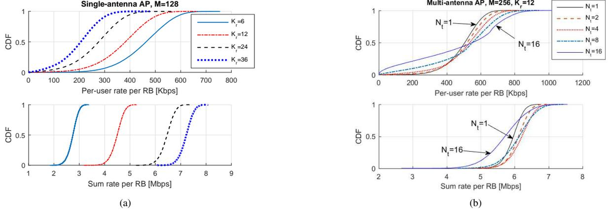
Fig. 2. Performance comparison with respect to the CDFs of per-user and sum data rates over a single RB. Part (a) utilizes  $M = 128$  single-antenna APs and the number of users varies from  $K_r = 6, 12, 24$ , to  $36$ . In part (b), a total of  $M = 256$  antennas are distributed over a set of multi-antenna APs (with  $N_t = 1, 2, 4, 8$  or  $16$ ) to serve  $K_r = 12$  users.
