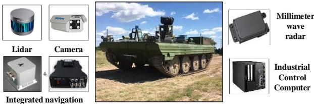
Figure 6. The unmanned tracked vehicle
