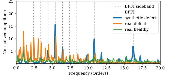
Fig. 4. CWRU normalized full-wave rectified envelope spectrum of an inner ring defect example with corresponding defect ball pass frequency (BPF) denoted by the dashed vertical lines. The difference between the real and synthetic fault in BPF frequencies and sidebands (shown by vertical dotted lines) motivates the use of domain adaptation.
