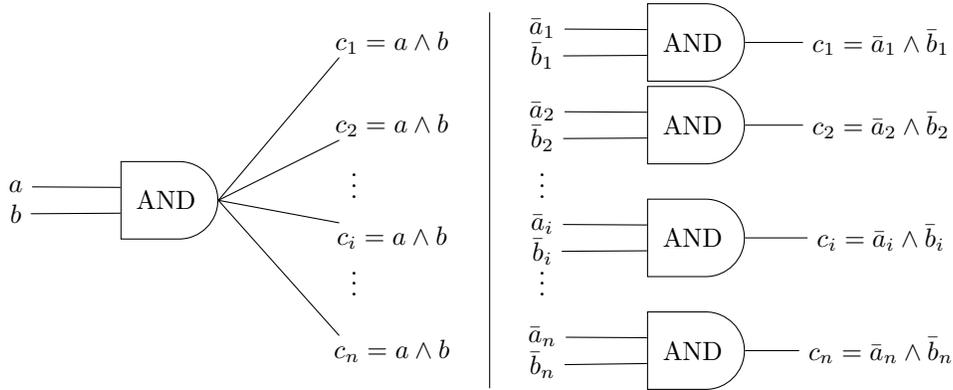
Figure 1: The left-hand side shows an AND gate with fan-out  $n$ . The right-hand side is its bounded fan-out equivalent. Here  $\bar{a}_i = a$  and  $\bar{b}_i = b$ . Gates of unbounded fan-out can be implemented with bounded fan-out as long as sufficient copies of the inputs are provided.
