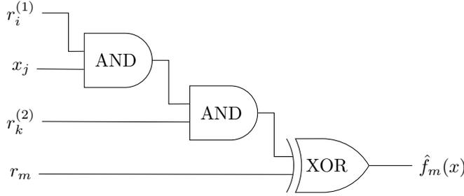
Figure 8: The circuit for evaluating each entry in the randomized encoding  $\hat{f}$ . The circuit shown here computes the  $m$ 'th entry, with  $m \leq k$ , consisting of the monomial  $r_i^{(1)}x_jr_k^{(2)}$  xored with  $r_m$ . For the entries with  $m > k$ , note that a single XOR gate is required.
