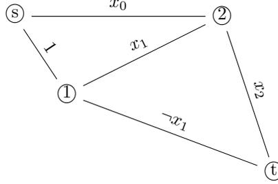
Figure 7: This size-4 mod-2 branching program consists of 5 edges whose connectivity is decided by the value of the input bits. Note that  $\neg x_1$  means that this edge is available if and only if  $x_1 = 0$ . As an example, when the input  $x = (x_0, x_1, x_2) = (0, 1, 1)$ , there is only one path from  $s$  to  $t$  which is  $s - 1 - 2 - t$ . Thus the output of this mod-2 BP will be 1.
