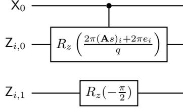
Figure 4: The quantum circuit for the vector addition operations in phase encoding. Here  $X_0$  is the first qubit of the  $X$  register that stores information of  $b$ .  $Z_{i,j}$  is the  $j$ 'th qubit of the  $i$ 'th GHZ state which stores information of  $\phi_i$ .
