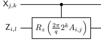
Figure 5: Part of the quantum circuit for matrix-vector multiplication in phase. Here  $X_{j,k}$  is the qubit that stores the  $k$ 'th bit of  $x_j$ , and  $Z_{i,l}$  is the  $l$ 'th qubit of the GHZ state storing the information of  $|\phi_i\rangle$ .
