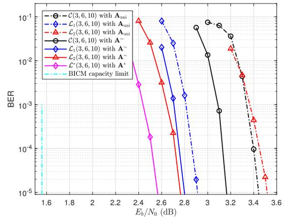
Fig. 6. BER of protograph based SC-LDPC coded uniform Gray labeled 16-QAM BICM with single-chain ensemble  $\mathcal{C}(3, 6, 10, 2)$  and connected-chain ensembles,  $\mathcal{L}_1(3, 6, 10, 2)$ ,  $\mathcal{L}_2(3, 6, 10, 2)$ , and  $\mathcal{L}^*(3, 6, 10, 2)$ , under the AWGN channel.
