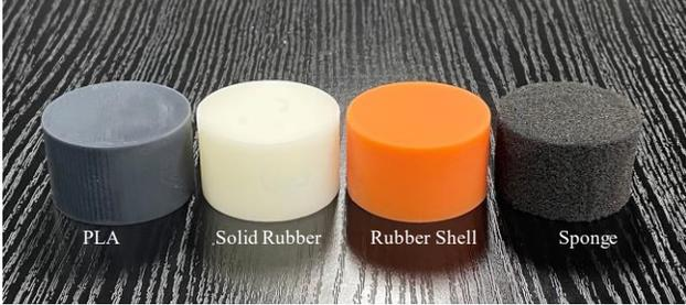
Fig. 4. The varied-stiffness cylinders for trial. An additional stiffness level of no contact is performed in the experiment.
