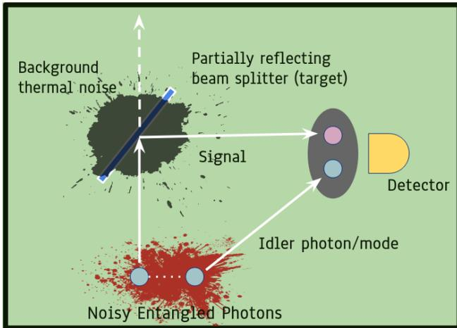
FIG. 1. A schematic representation of quantum illumination with noisy probes. The signal mode is sent towards the target, which is modeled by a weakly reflecting beam splitter. The idler mode is stored till the reflected signal comes back and the measurement is performed jointly on the two modes to infer the presence or absence of the target. The strong thermal background is always present, neighboring the target. Moreover, we consider different noise models in the probe states.
