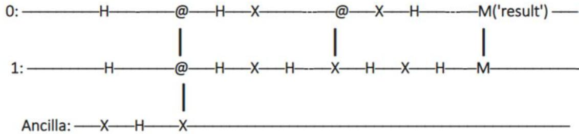
**Fig. 2:** Circuit for Grover's algorithm. @ symbol represents the control of the gates.
