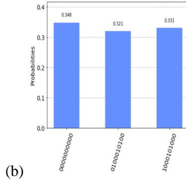
**Fig. 5:** (a) circuit for 10 qubit Grover's algorithm for finding darker pixel states and (b) the states located by Grover's algorithm
