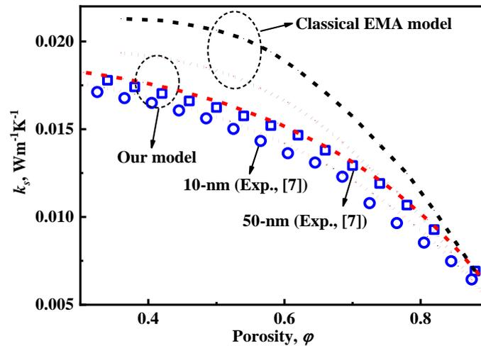
Fig. 2 Theoretical and experimental  $k_s$  comparison of the 10-nm and 50 nm NPBs.
