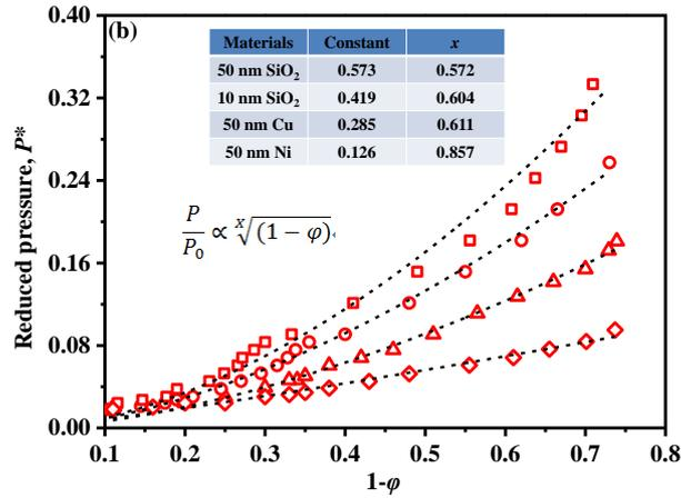
Fig. 1 Reduced pressure ( $P/P_0$ ) as a function of  $(1-\varphi)$ .
