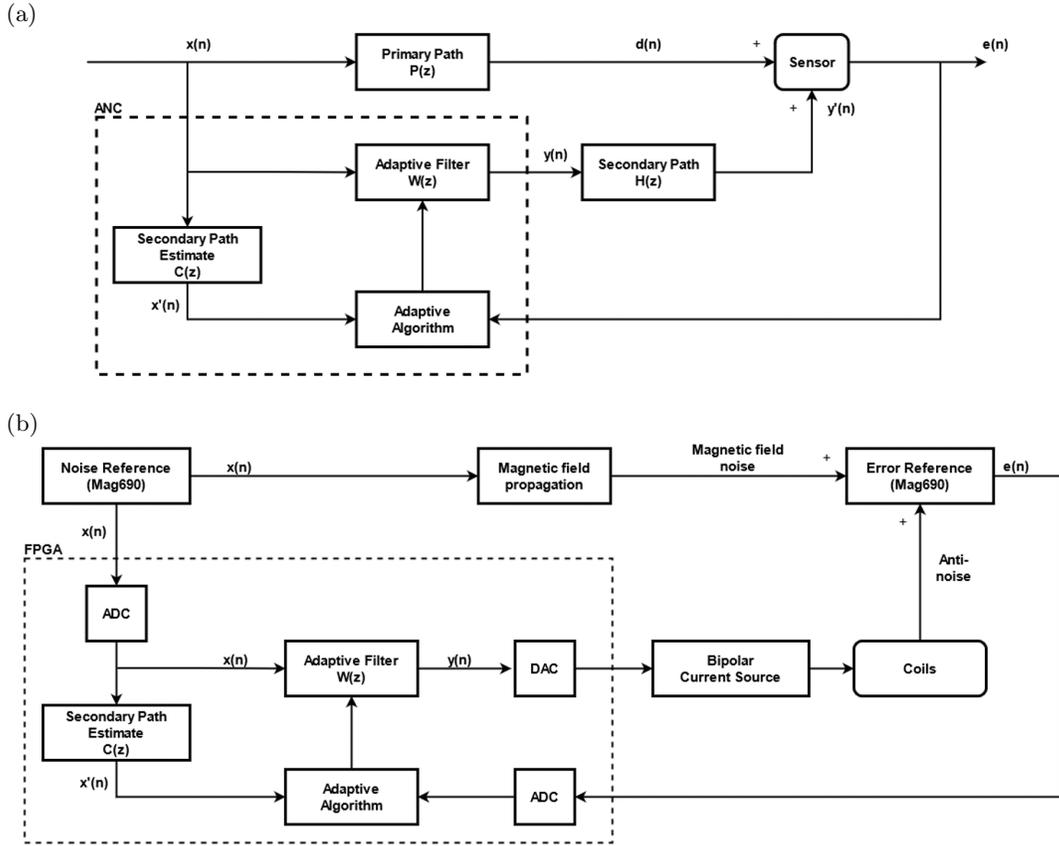
FIG. 3. (a) Theoretical structure of the primary and secondary paths. The ANC box contains the algorithmic elements of the adaptive filter that generates an anti-noise signal. Here we assume that the primary path  $P(z)$  transfer function does not have an appreciable effect on the signal detected at the sensor. (b) Experimental structure of the primary and secondary paths in the context of magnetic field generation and measurement. The ANC algorithm is contained within the FPGA chip.
