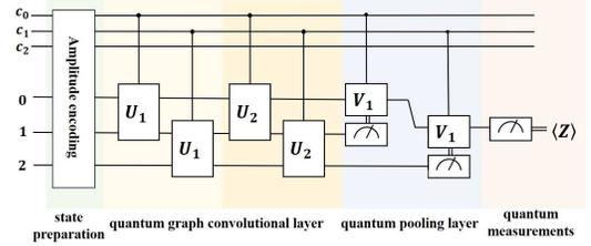
Fig. 4: A QGCN quantum circuit model
