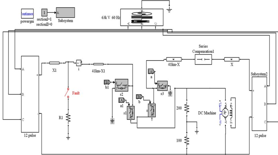
Fig.2. Total model of fault and railway
