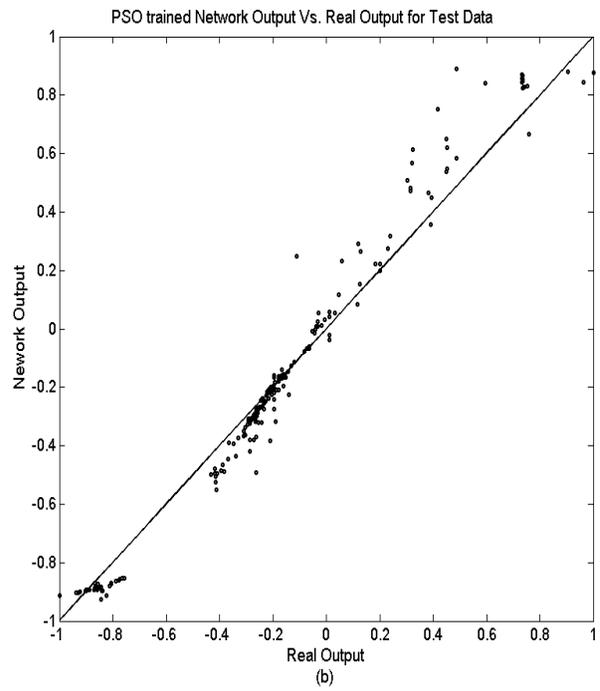
Fig.7. PSO trained Neural Network output vs. real output for a) train data b) test data
