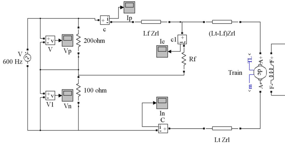
Fig.3. 600Hz Component circuit with train position beyond the fault location.
