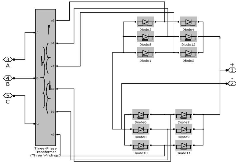
Fig.1. Tarsnsformer and 12 pulse rectifire
