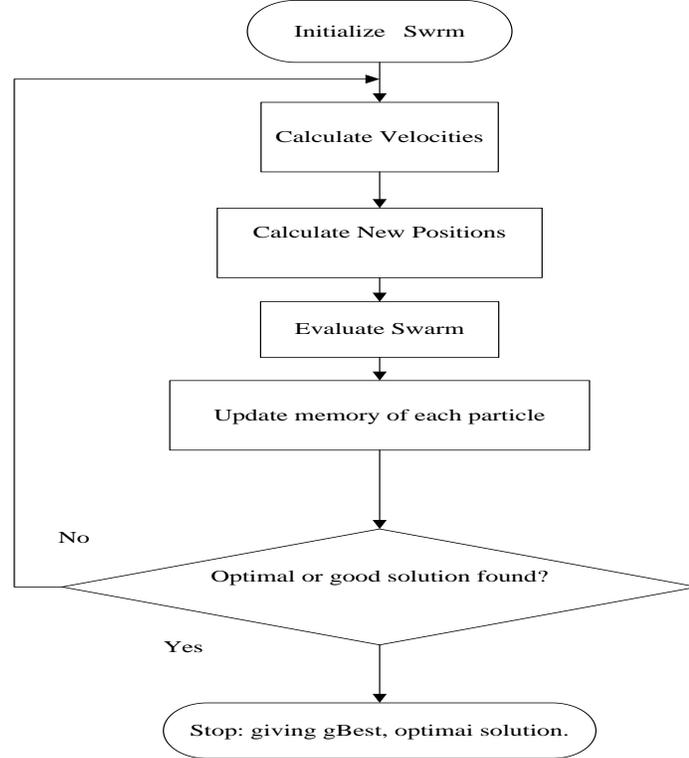
Fig.5. Flow chart for Particle Swarm optimization
