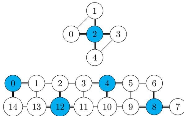
Fig. 5: *ibmq\_5\_yorktown - ibmqx2* (above) and *ibmq\_16\_melbourne* (below) qubit arrangements. For QACO implementation, the optimal position of the exploration qubits for UQAP problems are colored. Double lines represent the couplings between the ant and exploration qubits, single lines represent unused couplings.
