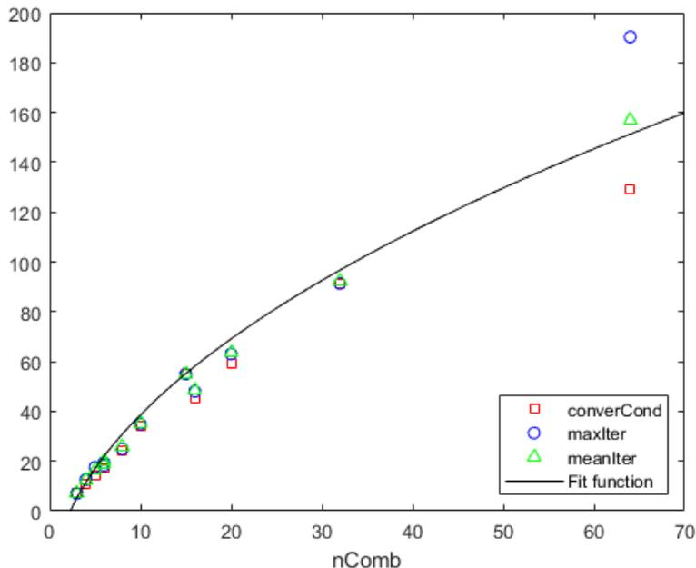
Fig. 4: Results for the parameter optimization. Mean iterations until convergence  $I_{term}$  (circle),  $converCondition$  (square) and  $MaxIter$  (triangle) vs  $nComb$ . The solid curve is the fitting curve for  $converCondition$  from equation 8.
