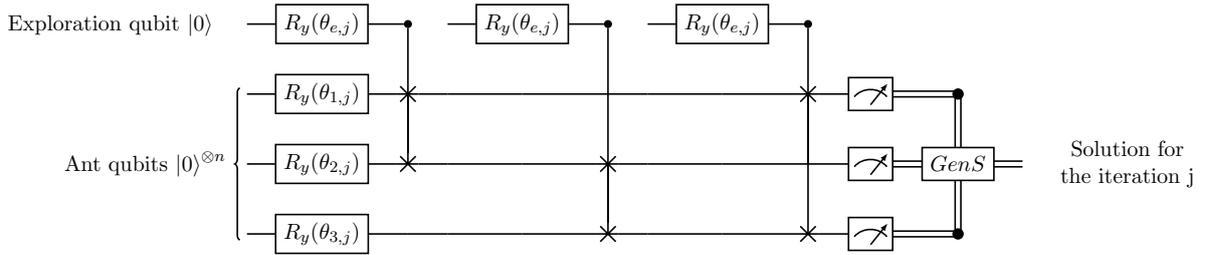
Fig. 2: Example of the diagram for the circuit that implements the  $j^{th}$  iteration of QACO for a constrained problem size  $n = 3$ . The pheromone update is made once the solution for the iteration is selected. The solution checking and conditional solution generation is shortened as “GenS”.
