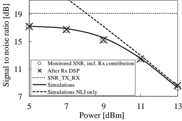
Figure 5 Signal-to-noise ratio obtained by spectral hole-based method (circles) accounting for the RX noise, constellation analysis of the received samples at the decision gate (crosses), and simulations (lines).
