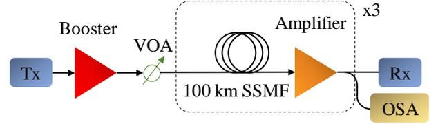
Figure 2: experimental set-up. VOA: variable optical attenuator, SSMF: standard single-mode fiber, OSA: optical spectrum analyzer. AWGN: additive white Gaussian noise.
