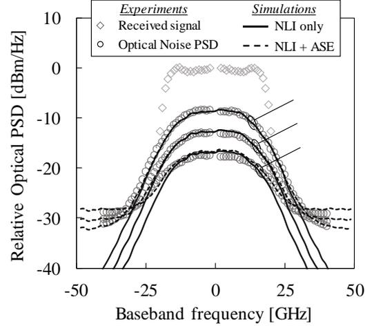
Figure 4: Experimental optical PSD of the RX signal (diamonds) and of the relative noise obtained with 1 GHz-wide spectral holes and for input power set to 9, 11 and 13 dBm (circles). Comparison with simulated relative optical PSDs in case of a pure NLI (solid lines) and a mixed NLI + ASE (dashed lines) impairments.
