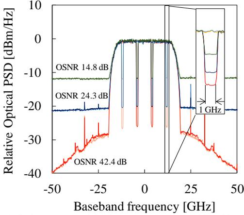
Figure 1: Relative optical PSDs (referenced to 0dBm/Hz for max spectral power) with different ASE noise levels for a 32.5 GBd signal with holes of width 1 GHz at  $\pm 4$  GHz and  $\pm 12$  GHz around the carrier frequency.
