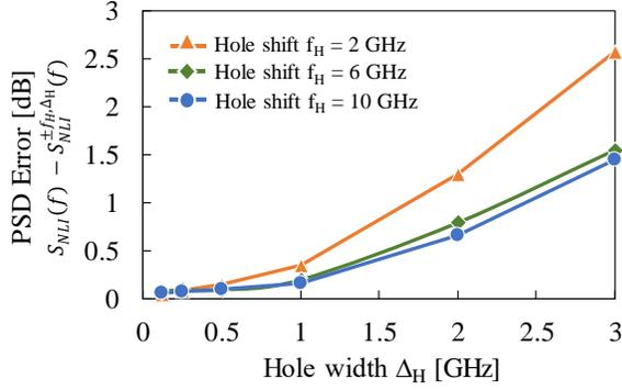
Figure 3 Variation of the PSD measurement errors with the spectral hole width for three different symmetric spectral hole positions respectively to the carrier frequency. Error is defined as the difference between the simulated PSD at the spectral hole position without and with a hole in the signal spectrum.
