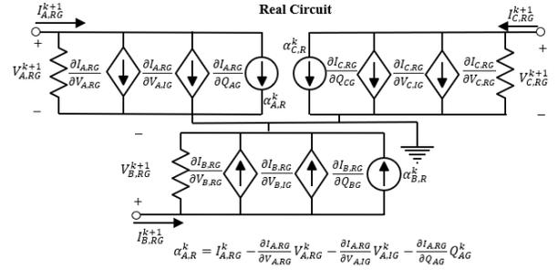
Fig. 1. Real circuit for a three-phase generator.  $\alpha_{B,R}^k$ , and  $\alpha_{C,R}^k$  are not shown.
