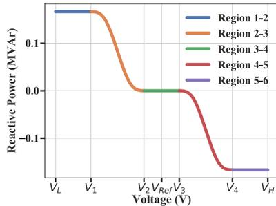
Fig. 3. Example piecewise Volt/VAR curve for an IBDG.
