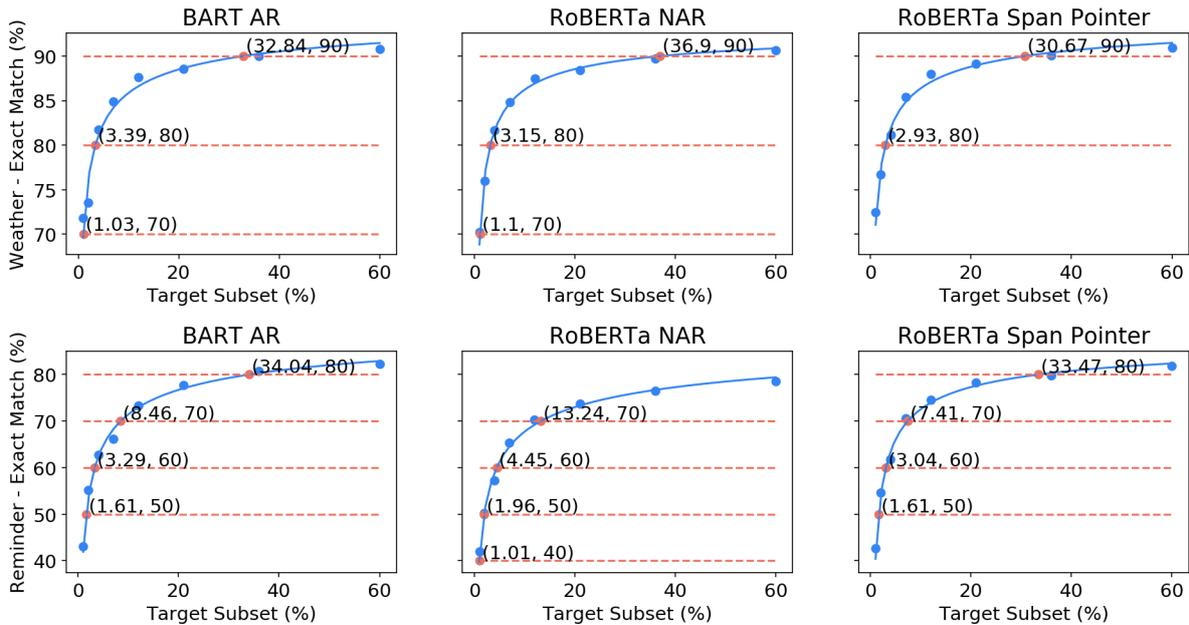
Figure 2: Data efficiency of various production-ready, transformer-based seq2seq parsers on the weather (top) and reminder (bottom) domains. The RoBERTa Span Pointer model is the most generalizable, achieving 90% exact match with 30.67% target data on weather and 80% exact match with 33.47% target data on reminder.
