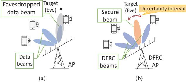
Fig. 1. (a) DFRC System imposed potential eavesdropper. (b) Secure DFRC system.
