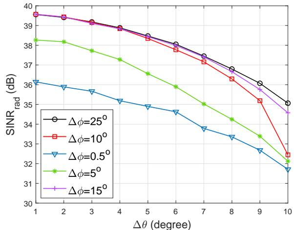
Fig. 9. Average SINR of radar versus angular interval of target location uncertainty,  $N_T = N_R = 10$ ,  $K = 5$ .
