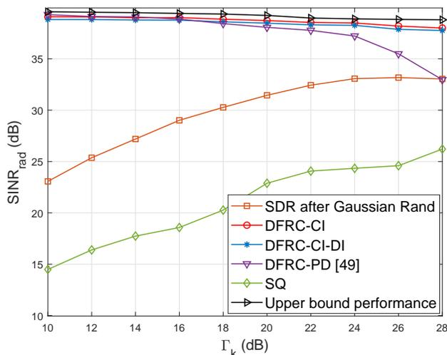
Fig. 7. The performance of radar SINR versus CU's SNR with different solving methods,  $N_T = N_R = 10$ ,  $K = 5$ .
