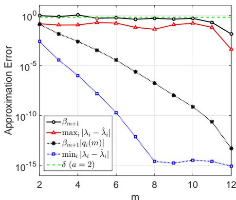
Fig. 4. Approximation error and upper bounds of the proximal EVD with thresholding when  $D = 12$ .
