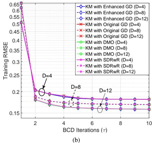
Fig. 3. Training RMSE vs. BCD iterations ( $\tau$  in Algorithm 4): (a) the artificial dataset (D1), (b) ML100K (D2).
