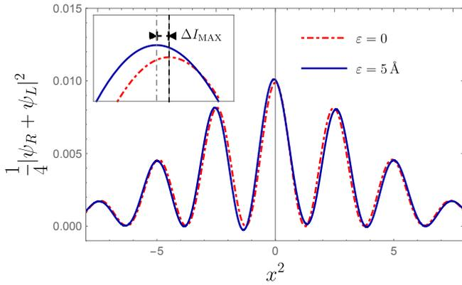
FIG. 2: Interference fringes pattern of a double-slit experiment in the presence of torsion generated by a screw dislocation (solid line) compared with the same setup in the absence of torsion (dot-dashed line).
