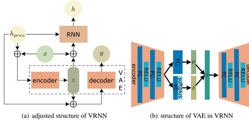
Figure 1: The core structure of CatVRNN.  $\oplus$  represents the concatenation of vectors. The VAE in the (b) figure is depicted in the (a) figure. FC denotes fully connected layer.  $\mu$  and  $\sigma$ , which are got by transforming the output of encoder, denote the mean and standard deviation of  $z$ , respectively.
