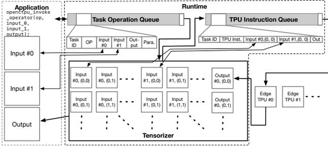
Figure 3: An overview of GPETPU's runtime system.
