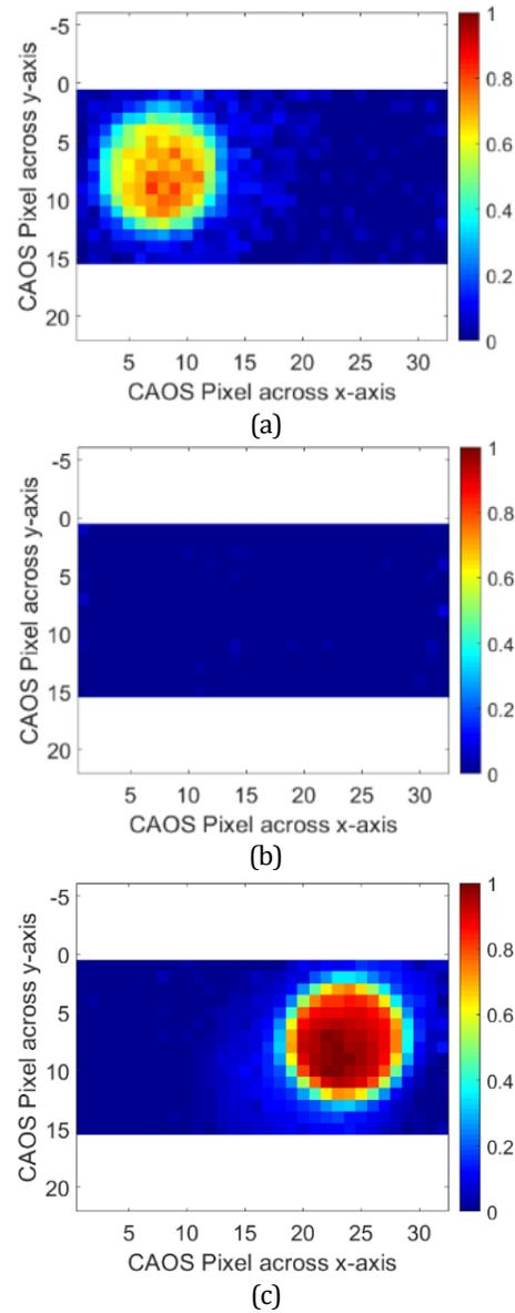
Fig.10. Target designed such that G-filter and B-filter imaged locations falling on DMD plane left and right sides, respectively. The independent and simultaneous FDMA-CDMA images are shown for (a) LED1 G-light at FM  $f_1=25$  KHz, (b) LED2 R-light at FM  $f_2=29$  KHz, and (c) LED3 B-light at FM  $f_3=35$  KHz.
