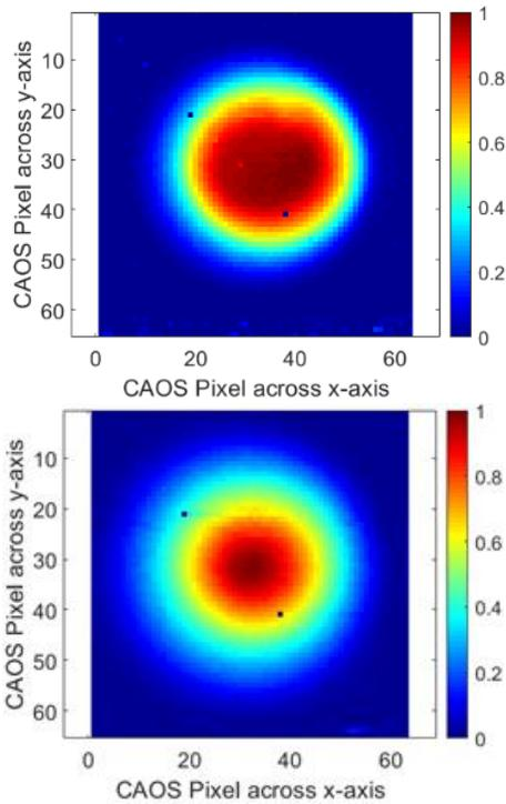
Fig.7. Top Image: 320-1000 nm CAOS image. Bottom Image: 800 - 1800 nm CAOS image. Both images shown in linear scale using passive FDMA-CDMA mode of the CAOS camera.
