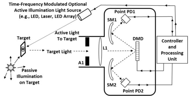
Fig. 1. Top view of the CAOS camera design for FDMA-CDMA mode operations for dual simultaneous spectral band operations. SM1/SM2: Spherical Mirrors; A1: Aperture; PD1/PD2: Different Material Large Area Point Detectors.
