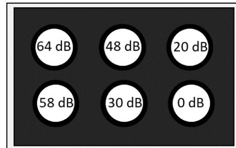
Fig.5 White light LED lightbox designed 6-patch 64 dB HDR test target.
