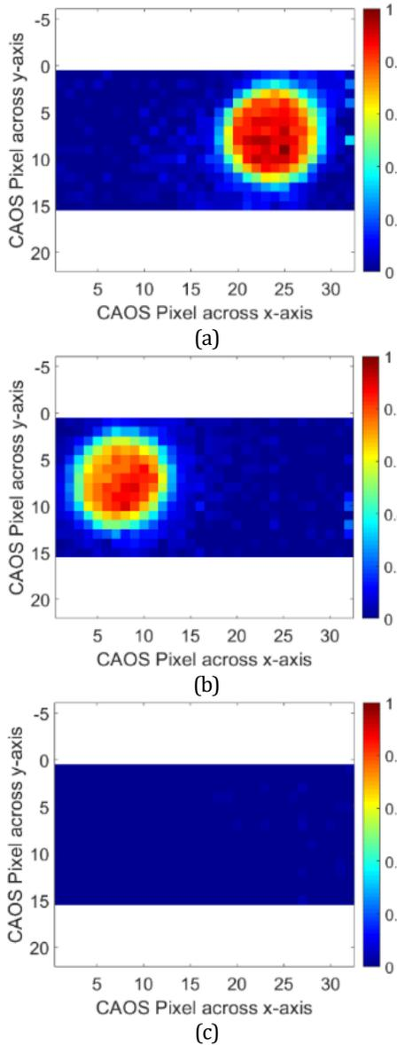
Fig.9. Target designed such that R-filter and G-filter imaged locations are falling on DMD plane left and right sides, respectively. The independent and simultaneous FDMA-CDMA images are shown for (a) LED1 G-light at FM  $f_1=25$  KHz, (b) LED2 R-light at FM  $f_2=29$  KHz, and (c) LED3 B-light at FM  $f_3=35$  KHz.
