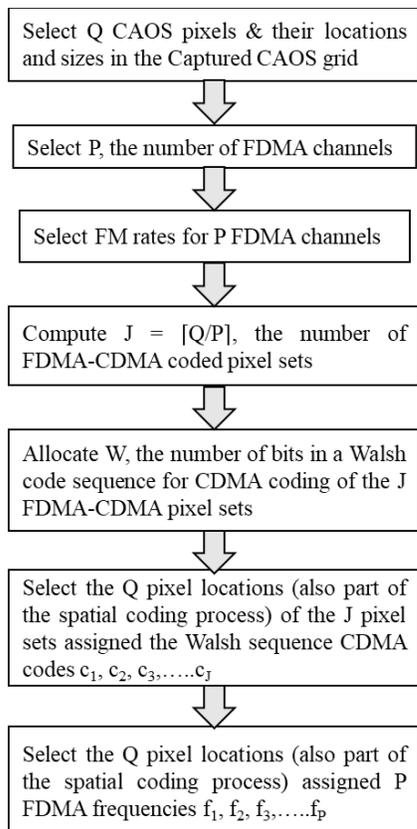
Fig.2. Flow chart for the CAOS space-time-frequency signaling FDMA-CDMA encoding operation per image frame.
