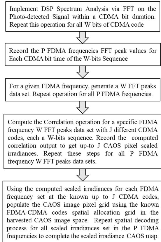
Fig. 4. Flow chart for the CAOS signal processing FDMA-CDMA decoding operation.
