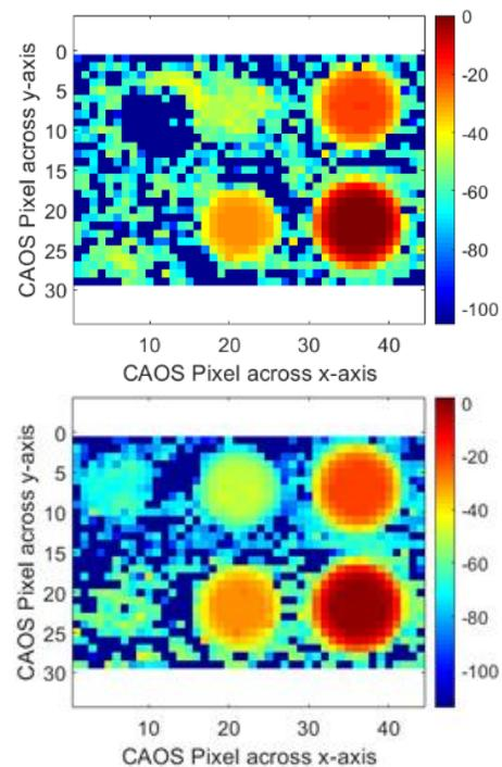
Fig. 6. (Top image) Passive FM-CDMA mode and (Bottom image) passive FDMA-CDMA mode CAOS camera measured DR dB scale images of the Fig.5 64 dB HDR target.
