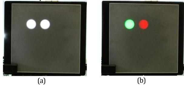
Fig.8. Room lighting photo of the deployed test target with 2 holes for testing the active FDMA-CDMA mode. (a) Target with open room white light lit holes and (b) Target with green and red optical filters placed on the 2 different holes.
