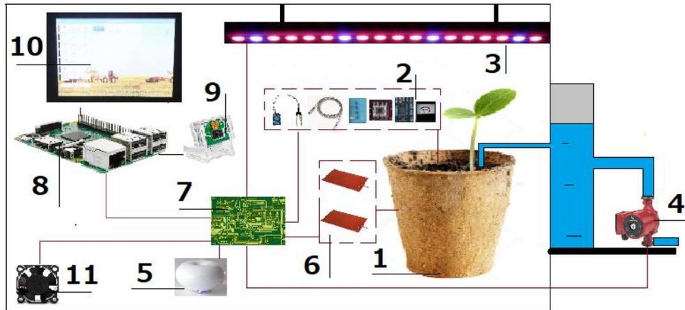
Fig.2. The farm operation scheme: 1 - crop, 2 - sensors, 3 - LED, 4 - pump, 5 - humidifier, 6 - air and soil heaters, 7 – analog digital converter, 8 - RaspberryPI, 9 - camera, 10 - operator panel, 11- fan.
