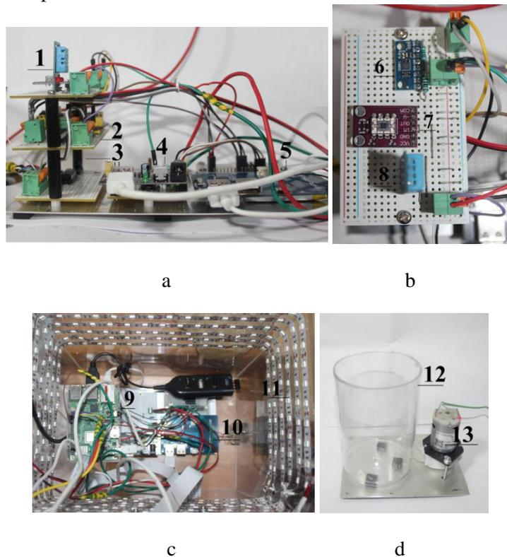
Fig. 3. Electrical part farm 1 - board with sensors, 2 ,3 - analog boards for signals processing, 4 - power board, 5 - battery, 6 - CO2 sensor, 7 - illumination sensor, 8 - temperature sensor, 9 - RaspberryPI3, 10 - battery board, 11 - LED, 12 - vessel for water, 13 - pump
