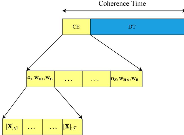
Fig. 2: Uplink training procedure for the hybrid RIS. We divide the coherence time in two sub-intervals, one for CE and the other for DT. We further divide the CE sub-interval into  $K$  blocks with each block containing  $T$  channel uses.
