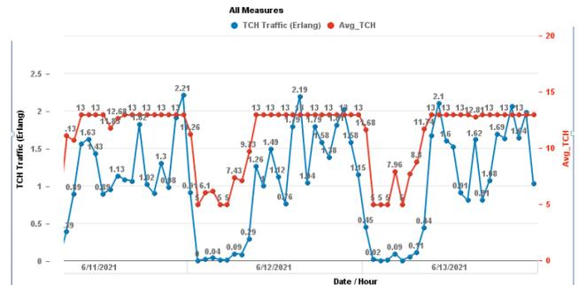
Figure 9: Traffic vs average TCHs for the same cell with power saving
