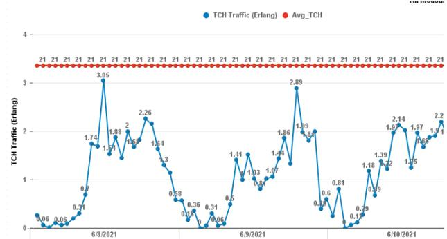
Figure 8: Traffic vs average TCHs for a cell without power saving
