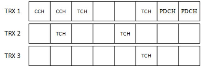
Figure 3: Mapping logical channels onto physical channels without BTS power saving.
