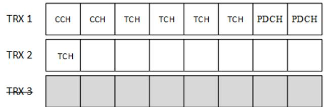
Figure 4: Mapping logical channels onto physical channels with BTS power saving.
