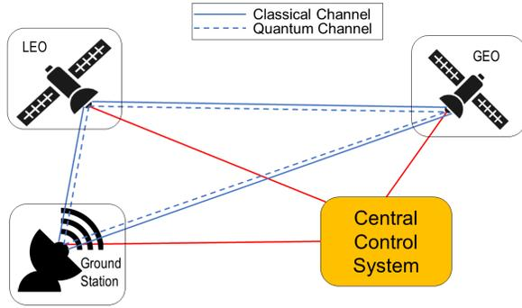
Fig. 1. Overview of the QKD network that combines GEO and LEO trusted-repeaters. The Central Control Unit knows the rate at which secret keys can be generated on the ground-to-space and inter-satellite quantum channels (dashed blue lines), determines the most convenient routing on the classical channels (solid blue lines) to optimize the flow of secret keys, and informs these decisions to the QKD nodes using the control channels (red solid lines).
