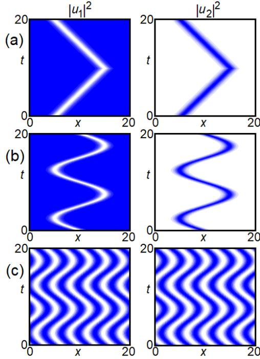
Figure 4: (a,b) Managed bright-dark vector soliton solutions (22) to the NLS system (19). We plot the square modulus of  $u_1$  and  $u_2$ , assuming (a)  $C(t)$  takes the form (8) with  $n = 2$ ,  $C_1(t) = t - T_1$ ,  $C_2 = -(t - T_1)$ ,  $T_1 = 10$ ,  $X_1 = 0.01$ ,  $x_0 = -15$  and (b)  $C(t) = -5 \sin(\pi t/5)$ ,  $x_0 = -10$ . (c) Managed cnoidal-snodal wavetrain solution (24) using  $C(t) = -2 \sin(\pi t/5)$ ,  $x_0 = -10$ . Colors are as indicated in Fig. 1.
