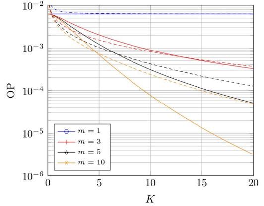
Fig. 4. OP comparison between fdRLoS (dashed lines) and Rician shadowed (solid lines) fading models. OP vs  $K$  for different values of  $m$ . Parameter values are  $\bar{\gamma} = 25$ dB and  $\gamma_{th} = 3$ dB.
