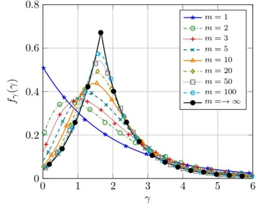
Fig. 1. PDF of the fdRLoS fading model for different values of  $m$  as a function of  $\gamma$  (in linear form). Parameter values are  $K = 5$  and  $\bar{\gamma}_{\text{dB}} = 3\text{dB}$ . Theoretical values (16) are represented with lines. Markers correspond to MC simulations. The case  $m \rightarrow \infty$  is the dRLoS PDF in [6, eq. (15)].
