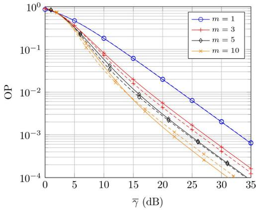
Fig. 3. OP comparison between fdRLoS (dashed lines) and Rician shadowed (solid lines) fading models. OP vs  $\bar{\gamma}$  (dB), for different values of  $m$ . Parameter values are  $K = 6$  and  $\gamma_{th} = 3$ dB. Markers correspond to MC simulations.
