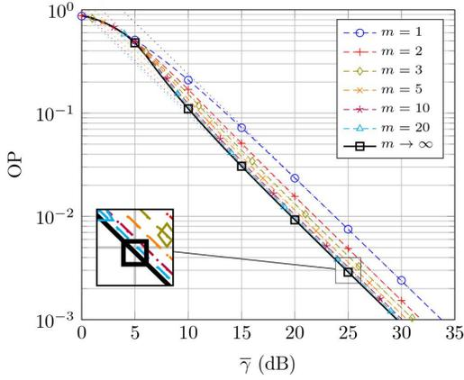
Fig. 2. OP plot. Parameter values are  $K = 1$  and  $\gamma_{th} = 3$ dB. Dashed lines correspond to fdRLoS fading. The case with  $m \rightarrow \infty$  corresponds to dRLoS fading [6, eq. (21)]. Dotted lines correspond to the asymptotic OP values in (21). Markers correspond to MC simulations.
