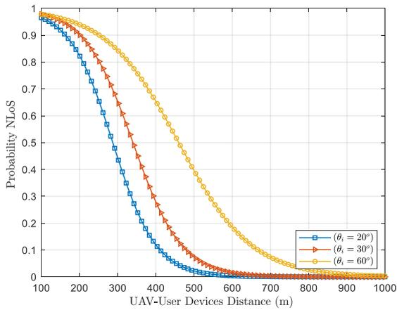
Fig. 3. Probability NLoS versus distance cross with different (Tethered angle ( $\theta_i$ )).
