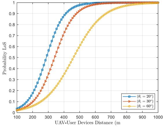
Fig. 2. Probability LoS versus distance cross with different (Tethered angle ( $\theta_i$ )).
