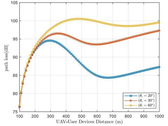
Fig. 4. Path loss versus distance cross with different (Tethered angle ( $\theta_i$ )).
