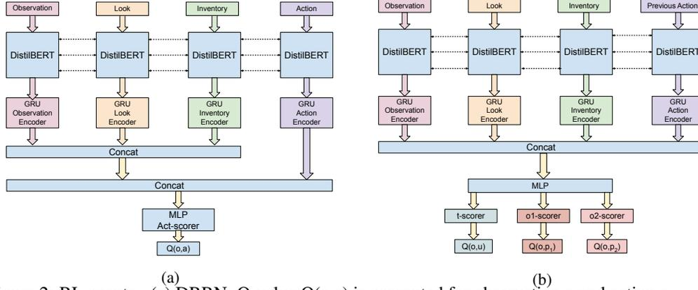
Figure 2: RL agents - (a) DRRN: Q-value  $Q(o,a)$  is computed for observation  $o$  and action  $a$ , (b) TDQN: Q-values  $Q(o,u)$ ,  $Q(o,p_1)$ ,  $Q(o,p_2)$  for all templates  $u \in T$  and all vocabulary  $p \in V$ .
