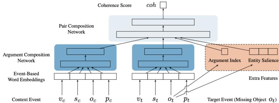
Figure 4: Cheng and Erk (2018)’s *event composition network* for computing a discourse coherence score between a context event and a target event. The illustration shows the target event’s direct object ( $o_t$ ) is the missing argument for this example.
