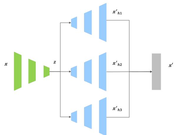
Figure 1. Multiple-hypothesis autoencoder architecture.
